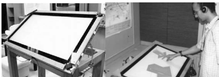
图9.1 MozArt公司桌面硬件原型。来源：Sharma A, Madhvanath S, Shekhawat A and Billingham M 2011。经授权转载
